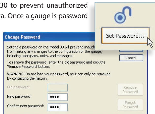
Figure 12 – Prevent unauthorized changes to a gauge with Password Protection.
