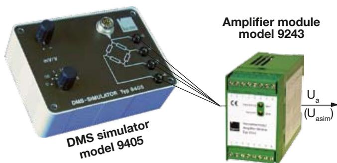
Given: SG sensor load cell model 8438-100 kN. Sensitivity of the sensor (acc. to calibration certificate) 1.678 mV/V. Amplifier output signal at nominal load 100 kN: U<sub>a</sub> = 10 V.
