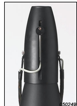
Fig. 1 Left: Top-view of Volume Velocity Adaptor showing phase-matched microphone arrangement. Right: Side-view of adaptor
