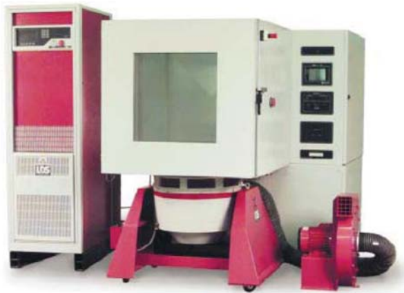
V830-SPA16K shaker system with an environmental chamber.
