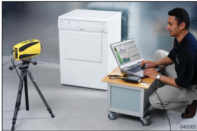
Fig. 1 Measuring on a washing machine with Type 8338
