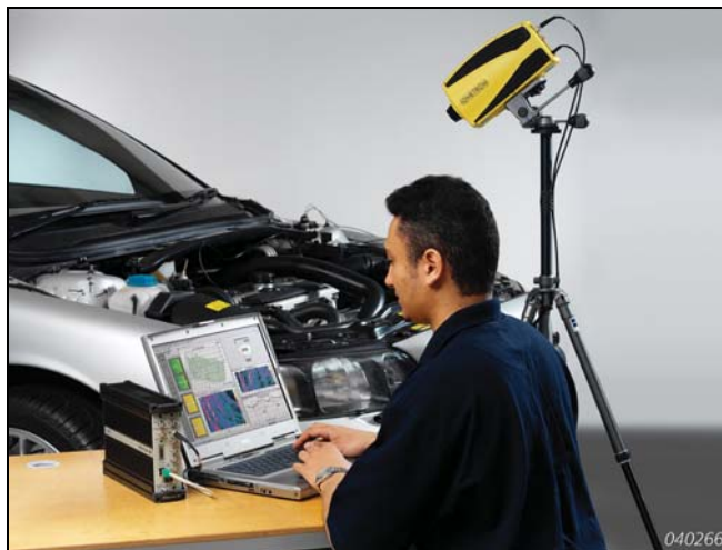
Fig. 2 Type 8338 connected to Type 3560-B PULSE Multi-analyzer for vibration measurement on a car engine
