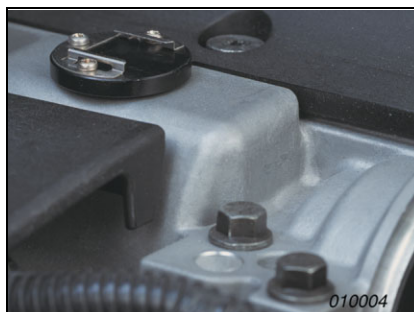
Fig. 4 High-temperature Mounting Clip UA 1563 Specifications: Temperature range: -55° to +175°C (-67° to +347°F) If discolouring can be accepted: -55° to +250°C (-67° to +482°F) Maximum acceleration: Perpendicular to mounting surface: 50 g peak Material: Base: Anodised aluminium; Spring: Stainless spring steel Weight: 11 gram
