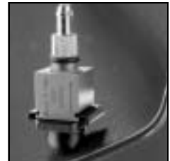
Fig. 8 Swivel Base UA 1478 mounted on a sloping surface with Type 4508
