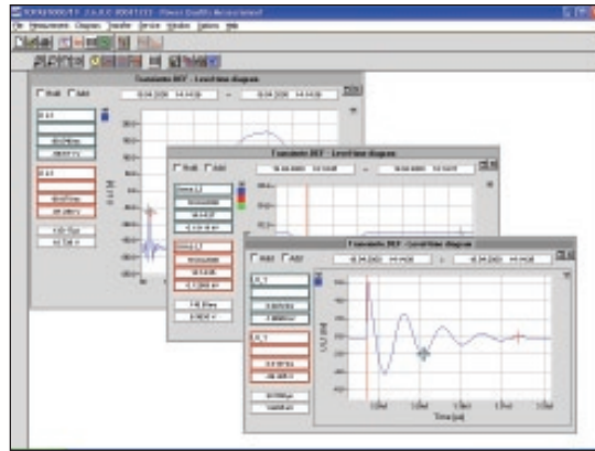
By double-clicking on an event, the software displays any trends and waveforms related to this event.
