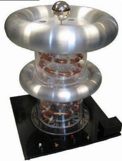
HVS with two 50 M sections for 100 kV
