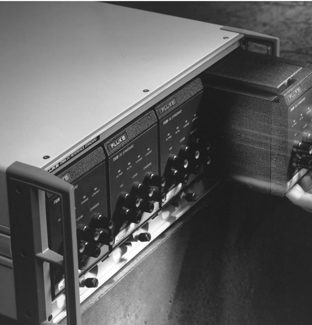
Because each 732B in the 734A Reference Standard is based on the same technology pioneered in the popular 732A—the first standards lab quality 10 V electronic reference—you can rely on it to provide the same high stability and predictable drift rate you’ve come to expect, in a smaller, more portable package.
