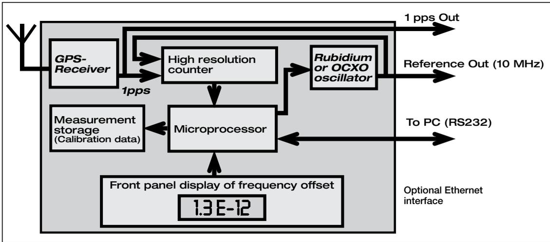
**Figure 2.** The Fluke 910 and 910R have built-in comparison between the GPS receiver and the internal oscillator. The frequency offset is displayed and stored and a traceability record can be produced at any time.
