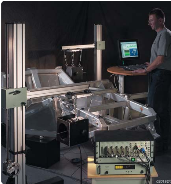
Fig. 11 Application of PULSE Multiple-Input Multiple- Output (MIMO) analysis using multiple shakers and accelerometers
