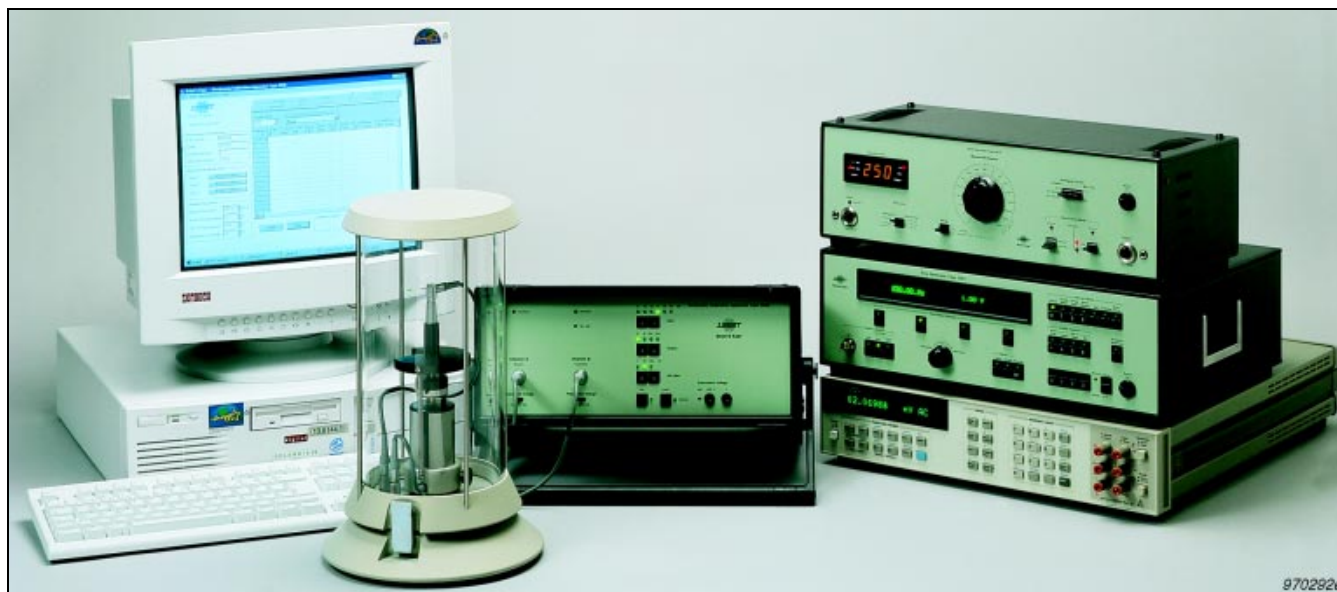
The main instruments of Reciprocity Calibration Apparatus Type 9699. From left to right and top to bottom, the controlling PC, Microphone Fixture UA 1412, Reciprocity Calibration Apparatus Type 5998, Band-pass Filter Type 1617, Sine Generator Type 1051 and a digital voltmeter
