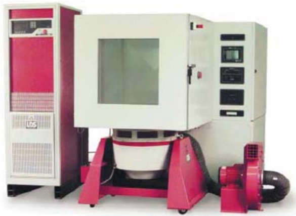
V830-SPA16K shaker system with an environmental chamber.
