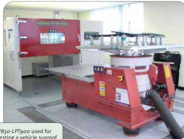
V850-LPT900 used for testing a vehicle sunroof in the vertical axis
