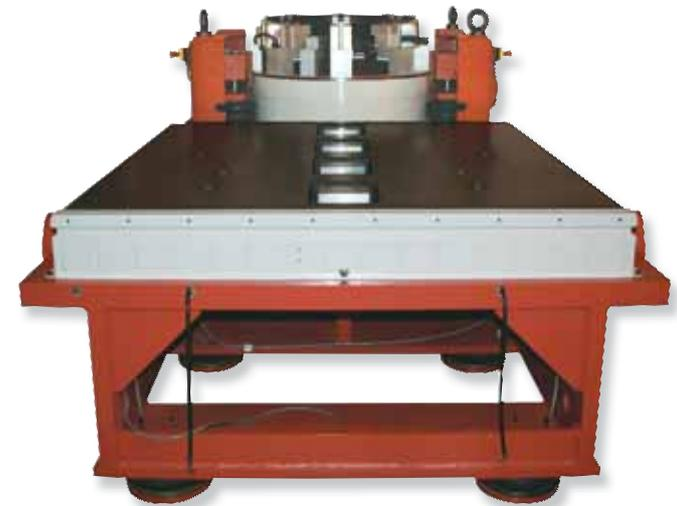
HBT Slip Table showing bearings along centre axis
