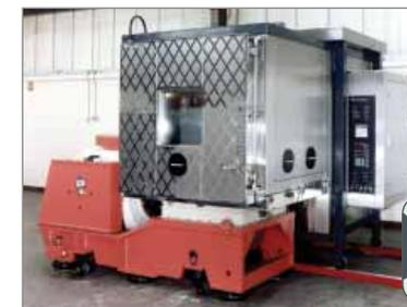
Combo system being used with an Environmental Chamber
