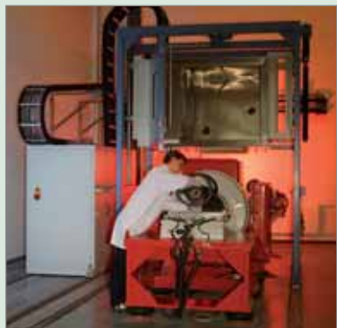
V9 mkII shaker with slip-table being set up for testing automotive components.
