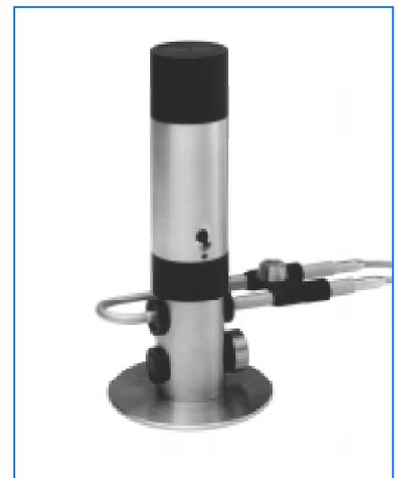
Fig. 6 Arrangement for measuring residual intensity and pressure-residual intensity index
