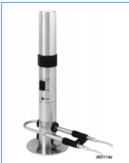
Fig. 4 Arrangement for sound pressure calibration
