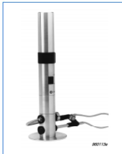
Fig. 5 Arrangement for sound intensity and particle velocity calibrations
