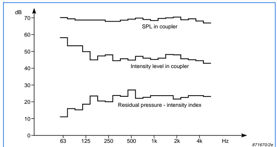
Fig.7 Intensity and sound pressure levels measured with the arrangement shown in Fig. 6. The pressure-residual intensity index spectrum is characteristic of the measurement system and is obtained by subtracting these two spectra
