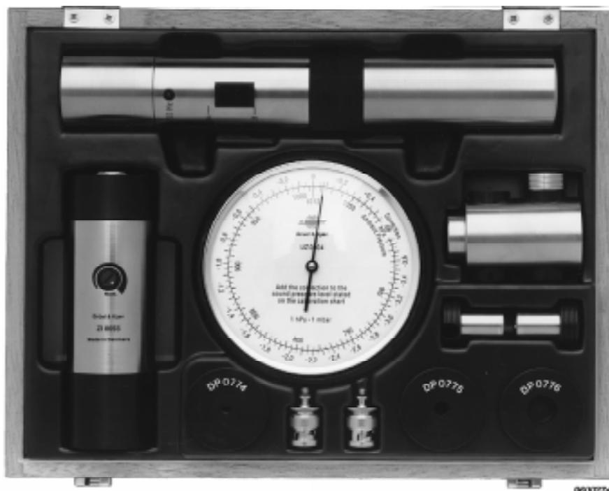
Fig. 1 Type 3541 components in their case. Main components: Intensity Coupler, Pistonphone, Sound Source. Other components: Correction Barometer, Dummy Microphone,  $1/4$ " Microphone Adaptors (two), Microphone Adaptors for Pistonphone ( $1/2$ ",  $1/4$ " and  $1/8$ "), 10–32 UNF to BNC Adaptors (two). In lid: Calibration Charts, Electrical Output Cables
