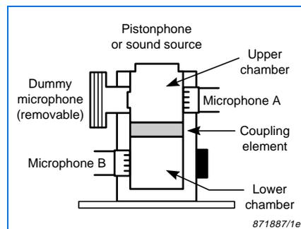
Fig. 2 Simplified cross-section of intensity coupler
