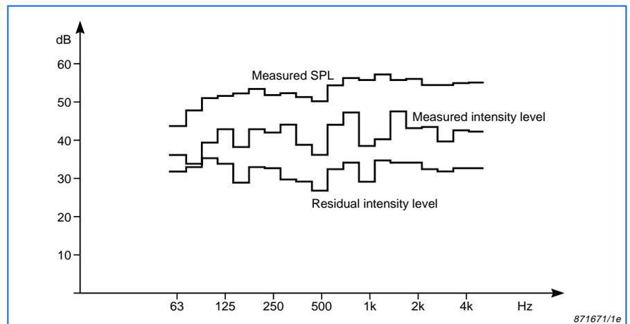
Fig.8 Sound intensity and mean sound pressure spectra measured in the field with an instrument calibrated with Type 3541. The residual intensity spectrum is obtained by subtracting the pressure-residual intensity index spectrum in Fig. 7 from the measured SPL spectrum
