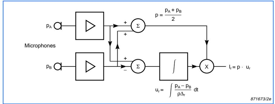
Fig. 3 Simplified block diagram of an intensity measuring instrument. The signals from two pressure microphones,  $p_A$  and  $p_B$ , are used to determine the pressure at the midpoint on the probe axis,  $p$ , and the particle velocity along the probe axis,  $u_r$ . Multiplying  $p$  and  $u_r$  gives the intensity reading  $I_r$ .  $\Delta_r$  is the microphone spacing and  $\rho$  is the density of air
