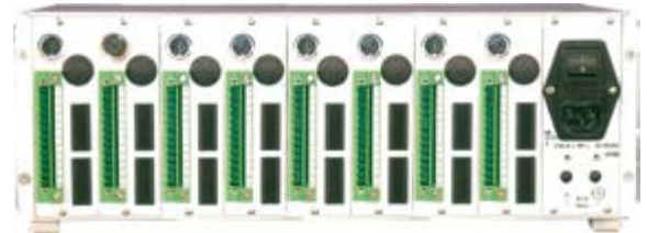
Back view: All sockets for sensors, control signals and serial interfaces are completely installed.
